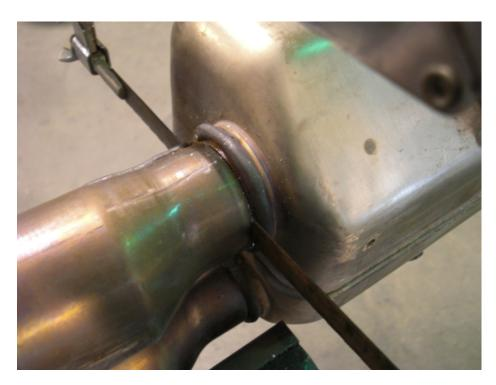
Stabilize the system in a bench vice. Make your cut as close to weld as possible.
