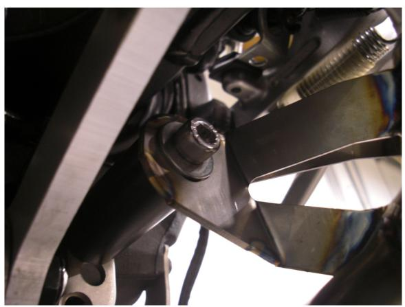
Re-attach O2 sensor and tighten all mounting hardware. The cables that actuated the valve in your stock muffler can be followed up to the servo motor and completely removed from the motorcycle, or, you may tuck them out of the way somewhere and zip tie them to the chassis.
